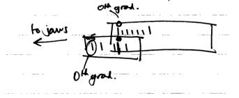
The extreme end of the second scale towards the jaws denotes -0.5 so will not be lined up with the  $0^{th}$  grad of the main scale 12.
